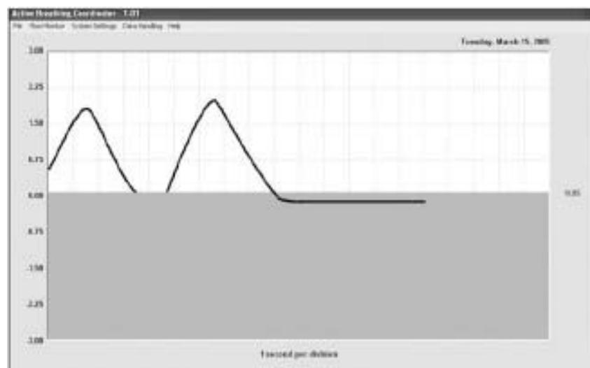
Figure 1: Active Breathing Coordinator screen display where exhale breath hold is triggered, as shown by the flat line.
