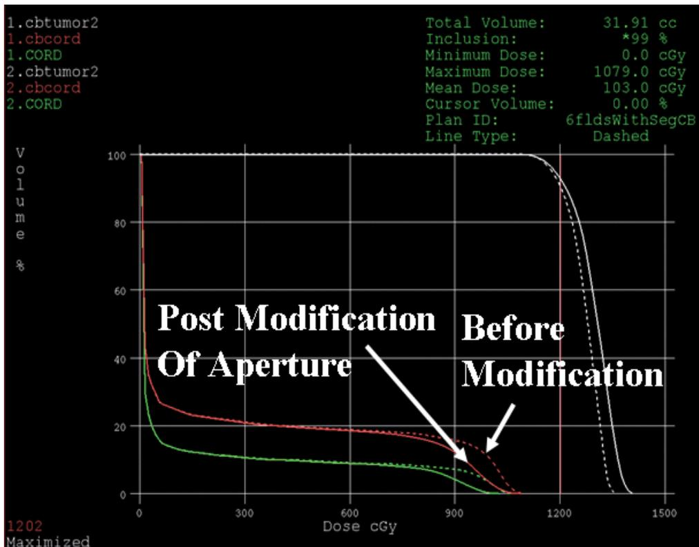
By making minor changes to the leaves along the spinal cord, the dose to this critical structure was reduced to agree with the original dose constraints. This can be seen in the DVH shown above.
